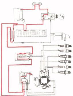
Group 39 Wiring diagrams 260/1978 The electronic module interrupts current flow, ignition coil discharges (sparks) through the secondary winding.
